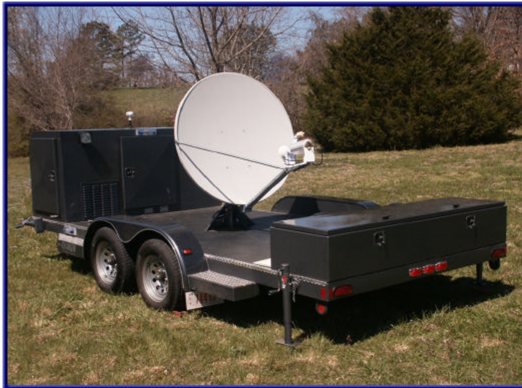
Trailer with a 1.2m Satellite Antenna.
